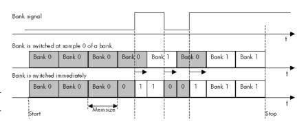
The data of the two different output signals are stored in multiplex format. For this reason the output signal on the dedicated channel is only updated with half of the programmed sample rate, when bank switching mode is enabled.
