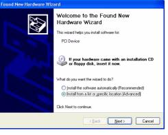
Allow Windows XP to search for the most suitable driver in a specific directory. Select the CD that was delivered with the board as installation source. The driver files are located on CD in the directory
