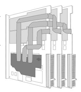
As some of the synchronization cables are not secured against wrong plugging you should take care to have the pin 1 markers on the multiple connectors and the cable on the same side, as the figure on the right is showing.
