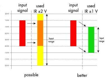
The example in the right figure shows signals with a range of  $\pm 1.0$  V that have offsets up to  $\pm 1.0$  V. So related to the desired input range these signals have offsets of  $\pm 100$  %.
