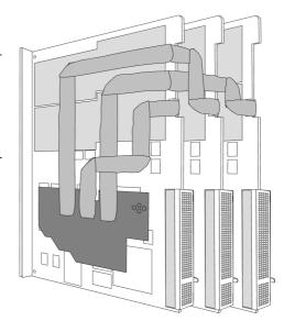
As some of the synchronization cables are not secured against wrong plugging you should take care to have the pin 1 markers on the multiple connectors and the cable on the same side, as the figure on the right is showing.
