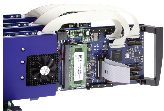
Image 9: M4i cards with star-hub ex installed and connecting cables
