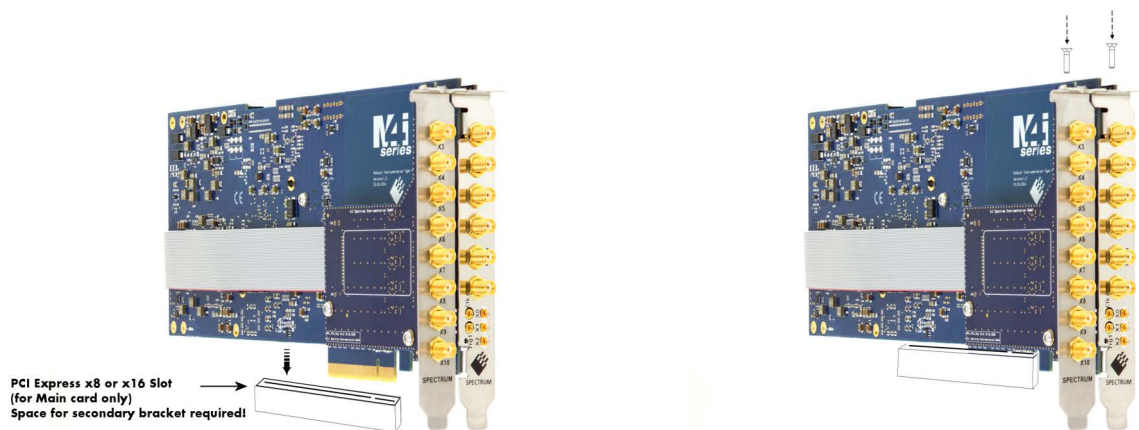
Image 7: M4i card with digital option mechanical installation and position of screws
