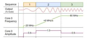
Above, the example sequence of three commands for a single core, shows a fixed 20 MHz frequency with 60% amplitude in step 1, a 10 seconds frequency ramp with 6 MHz/s slope and full 100% amplitude in step 2 and finally, in step 3, a fixed 80 MHz frequency with 50% amplitude. Each step consists of only 3 to 4 single line commands to set the mode, frequency, amplitude and timing.
