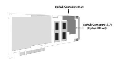
tween the different cards. The figure shows the piggy-back module mounted on the base board schematically without any cables to achieve a better visibility. It also shows the locations of the available connectors for the two different versions of the star-hub option.
