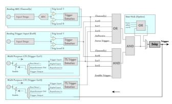
All of the Spectrum M3i series cards allow the user to program an additional trigger delay. As shown in the trigger overview section, this delay is the last element in the trigger chain. Therefore the user does not have to care for the sources when programming the trigger delay.
