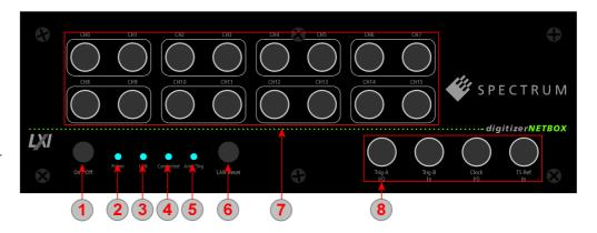
In area 8 a version with 4 BNC connectors is shown. Other versions with 5 SMA, 6 BNC or 7 SMA connectors are also available. Please see the table below for the different connections.
