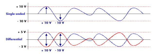
As you can see in the block diagram mentioned earlier in this manual, the internal conversion from differential to single ended is done after the offset correction stage. As a result all the offset settings mentioned before can only be used with single-ended inputs.
