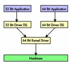
After installation of the Spectrum 64 bit driver there are two general ways to access the hardware and to develop applications. If you're going to develop a real 64 bit application it is necessary to access the 64 bit driver dll (spcm\_win64.dll) as only this driver dll is supporting the full 64 bit address range.
