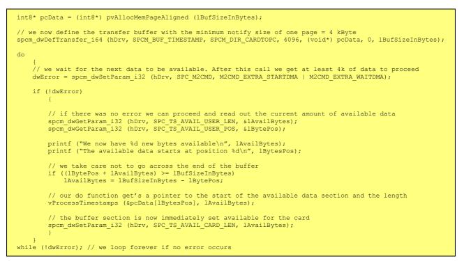
The extra FIFO has a quite small size compared to the main data buffer. As the transfer is done initiated by the hardware using busmaster DMA this is not critical as long as the application data buffers are large enough and as long as the extra transfer is started BEFORE starting the card.
