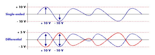
As you can see in the block diagram mentioned earlier in this manual, the internal conversion from differential to single ended is done after the offset correction stage. As a result all the offset settings mentioned before can only be used with single-ended inputs. You can change between single-ended and differential mode separately for every input channel by setting the relating register shown in the following table:
