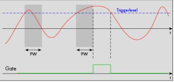
The pulsewidth trigger modes for long pulses can be used to prevent the board from triggering on wrong (short) edges in noisy signals.
