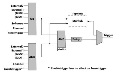
All analog D/A and A/D cards have one external trigger input (External0) and digital i/o cards and pattern generators have one to two external trigger inouts (External0 and External1). In addition using the option BaseXIO it is possible to have two additional trigger inputs named XIO0 and XIO1 in the drawing.
