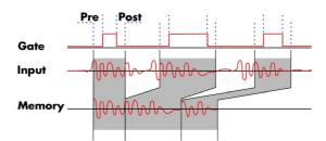
When using Gated Sampling the maximum pretrigger is limited as shown in the technical data section. When the programmed value exceeds that limit, the driver will return the error ERR\_PRETRIGGERLEN.
