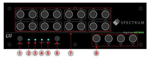
In area 8 a version with 4 BNC connectors is shown. Other versions with 5 SMA, 6 BNC or 7 SMA connectors are also available. Please see the table below for the different connections.
