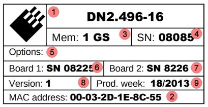
The Spectrum type plate, which consists of the following components, can be found on the back of all netbox products. Please check whether the printed information is the same as the information on your delivery note. All this information can also be read out by software:
