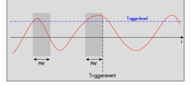
The pulsewidth trigger modes for long pulses can be used to prevent the board from triggering on wrong (short) edges in noisy signals.
