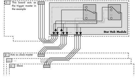
the trigger events, if all synchronized cards run with the same sampling rate. Any one of the synchronized cards can be used as a clock master and besides any card can be part of the trigger generation.
