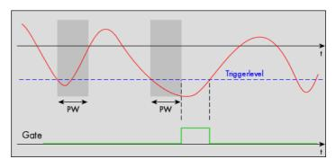
The pulsewidth trigger modes for long pulses can be used to prevent the board from triggering on wrong (short) edges in noisy signals.
