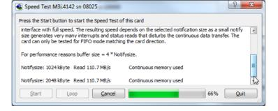
Repetitive Memory Transfers: single DMA data transfers are repeated and measured. This test simulates the measuring of pulse repetition frequency when doing multiple single-shots. The test is done using different block sizes. One can estimate the transfer in relation to the transferred data size on multiple single-shots.
