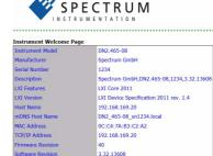
The integrated webserver follows the LXI standard and gathers information on the product, set up of the Ethernet configuration and current status. It also allows the setting of a configuration password, access to documentation and updating of the complete instrument firmware, including the embedded remote server and the webserver.
