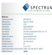
The integrated webserver follows the LXI standard and gathers information on the product, set up of the Ethernet configuration and current status. It also allows the setting of a configuration password, access to documentation and updating of the complete instrument firmware, including the embedded remote server and the webserver.
