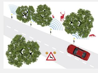
low power so Long Range Wide Area Network (LoRaWAN) is used as it can reach up to 40 km in rural areas. This standard is characterized by its low energy consumption, and is based on unlicensed frequency bands and therefore available at low cost.
