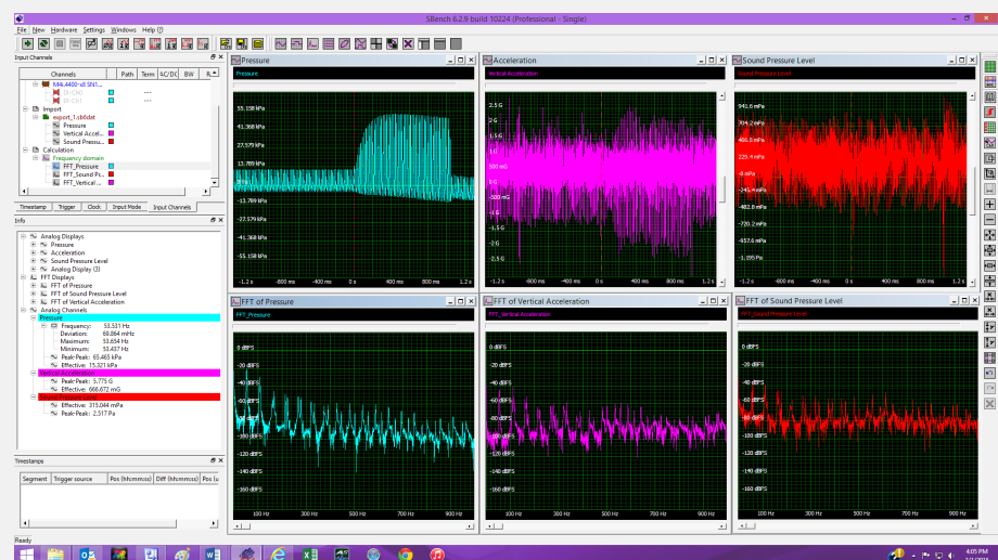
Figure 6: Measuring the pressure, vibration, and sound level of a small air compressor and showing the effect of blocking the output port. The top three grids show (from left to right) the pressure, vibration, and sound level with related FFT's shown below each.
