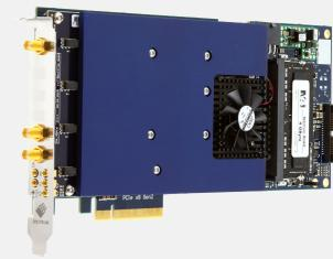
The Spectrum M4i.2230-x8 8 bit 5 GS/s PCle digitizer is used to acquire the RKE signals
