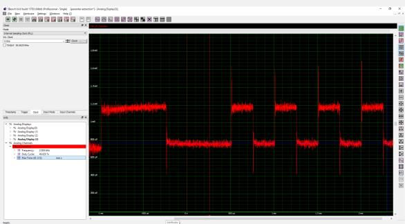
Figure 4: Measurements made on the demodulated FSK signal include the frequency, duty cycle, and rise time. The measurements are gated by the cursors and include only the four pulses on the right of the display.
